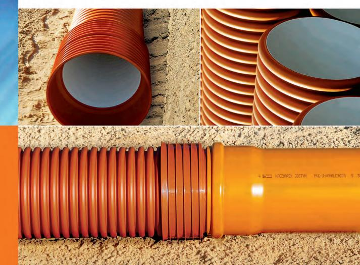
The comparison of cross-sections of a **structured type B pipe** whose nominal size refers to the inner diameter (DN/ID) and a pipe whose nominal size refers to the outer diameter (DN/OD) shows that the cross-section area of the former is on average 32% bigger than that of the latter. Thus K2-Kan pipes have a considerably bigger inner diameter than other pipes of the same nominal size based on the outer diameter.
