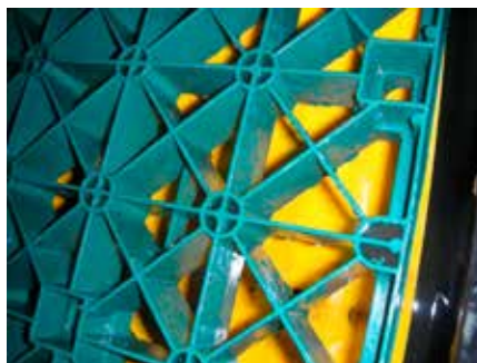
Cleaned, residue-free system; the area of the flow separator is displayed here
