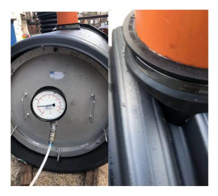
DN750 Twin-wall pipe x 110mm twin-wall lateral adaptor at 2bar
