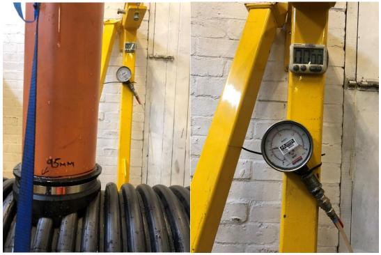
Result: No visible leaks after 15 minutes and no pressure drop on the guage.
