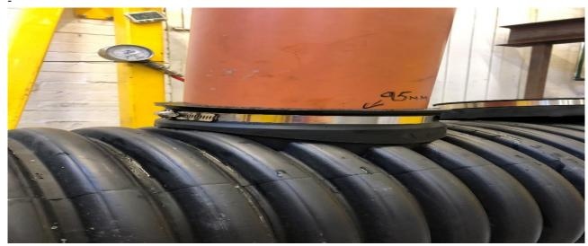
Pipe stoppers were fitted at either end of the pipe and to prevent these from dislodging, additional restraint in the form of wooden supports were used, these being held in place using strapping. A 160mm end cap was also held in place using strapping to prevent it being dislodged during the test.
